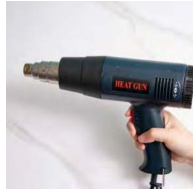
4. Heat the shrink film to make it fit tightly with the substrate;
