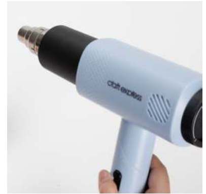
4. Heat the shrink film to make it fit tightly with the substrate;
