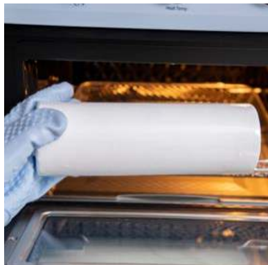
5. Print the substrate with sublimation oven.
