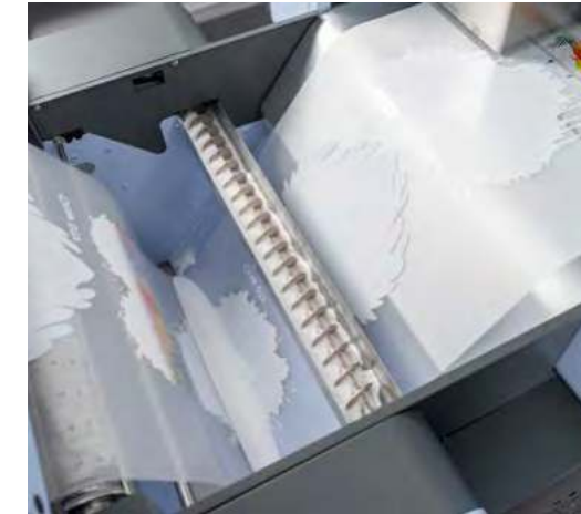
Auto Powder Recycling System It can effectively improve the utilization rate of hot melt powder and minimize waste. In addition, it saves the hassle of shaking powder by hand, allowing the powder to be spread more evenly on the film.
